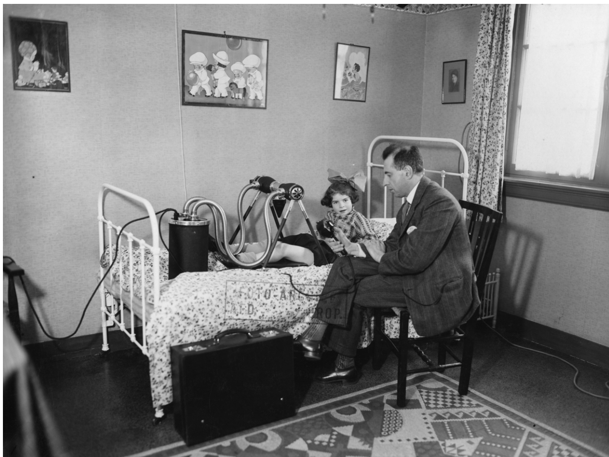
The Philips mobile Metalix, 1930. The Metalix Junior made it possible for doctors to make diagnoses at the bedside ©Philips Company Archives
